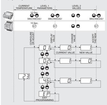
**ADJUSTMENT:** Pressing once the CONFIGURE OR ADJUST keys accesses the user's parameters adjustment. The proceeding is the same as for the configuration and access is only possible to the parameters defined as adjustable by the user in the configuration. In order to access the parameters the parameter 39 parameter should be configured.
